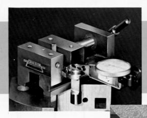
The picture at the left is an example of how the Criterion toolmaker's vise can be used as an inspection tool. The part being held is a flexure — a highly precision component of a valve for use in one of the newer missiles. This photo shows an inspection procedure using two parallel pins upon which the undersides of the flange rest. This permits checking flange thickness in relation to a reference point on a radius on the underside.
